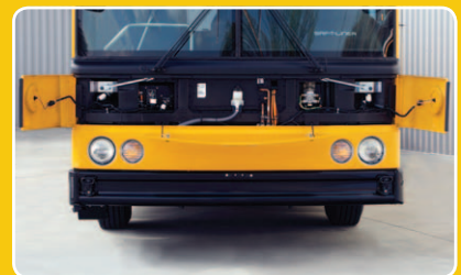
Full-width front access panel allows for easy access.
